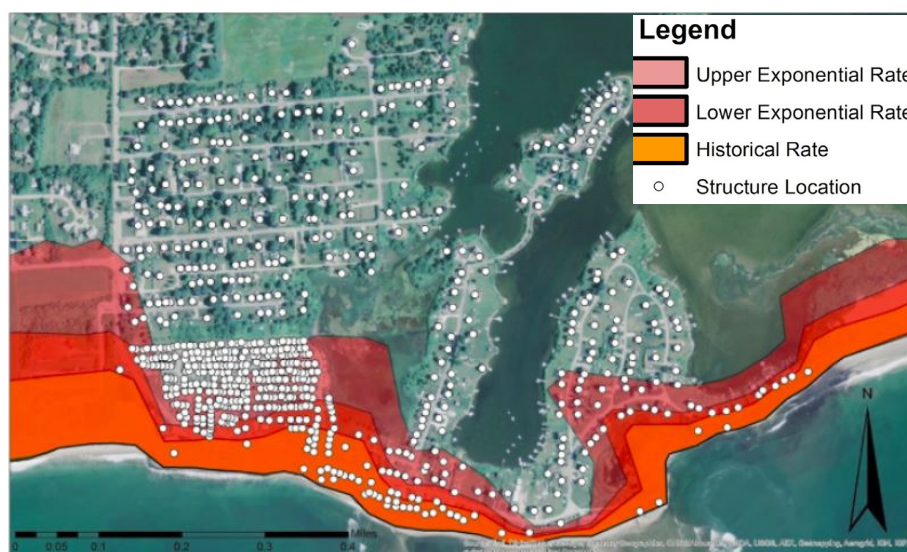
Figure 10. Estimated positions of the shoreline in the study area after 100 years using the historical erosion rate and two exponentially increasing erosion rates.
