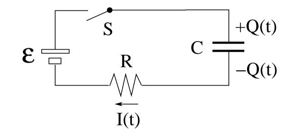
Physical properties of *RC* circuit during charging process determined by 3 combinations of the device properties:
