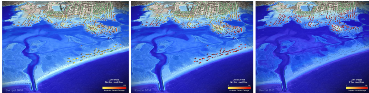
Figure 22. Three dimensional (3d) visualization of the percent damage to structures for Charlestown, RI: 100 year dunes intact (upper panel), 100 year dunes eroded (center panel), and 100 year dunes eroded, with 2.1 m (7 feet) SLR and shoreline erosion (lower panel). The lower panel projects coastal erosion to 2100.
