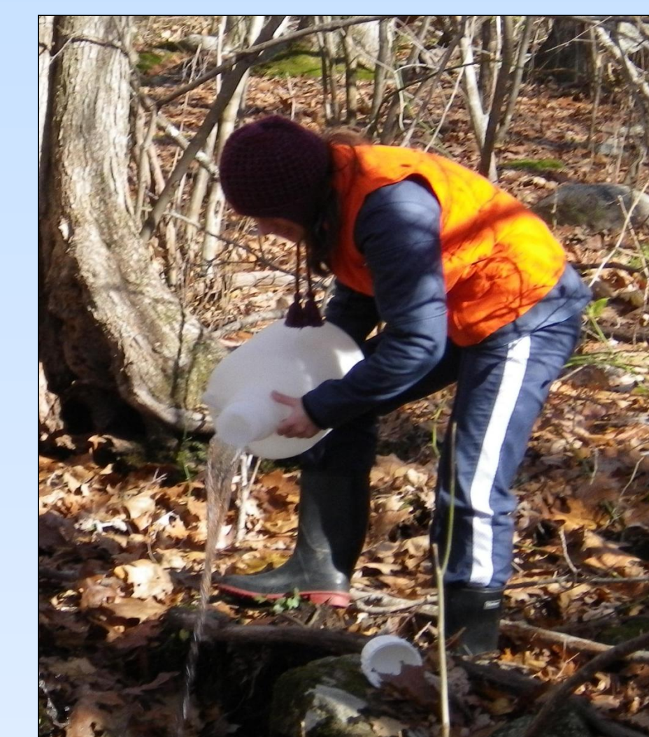
Figure 4: A slug containing amendments was introduced and sampled 30 m downstream
