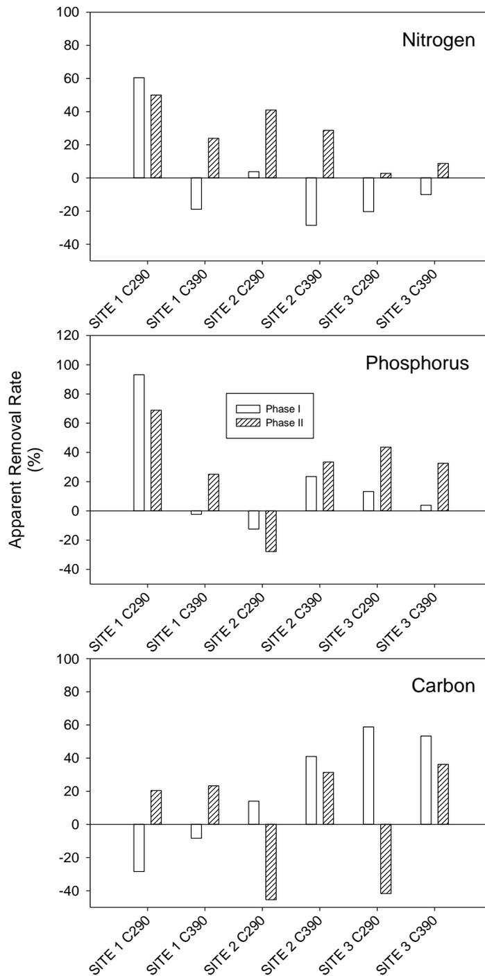
**Figure 5.** Actual removal rates for nitrogen, phosphorus and dissolved organic carbon at the three study sites prior to (Phase I) and during (Phase II) operation of intermittent soil aeration. Values are for lysimeters at 90 cm below the infiltrative surface placed between (C2) and downstream from (C3) leachfield trenches. Actual removal rates were calculated using Equation (2). Negative values indicate net constituent production.
