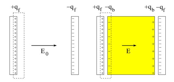
The bound surface charge has the effect of reducing the electric field between the plates from  $\vec{E}_0$  to  $\vec{E}$ .
