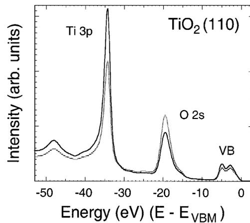
FIG. 2. Photoelectron spectra from the rutile  $\text{TiO}_2(110)$  surface recorded within the photon-energy width of the  $\text{TiO}_2(200)$  Bragg back-reflection condition. The photon energies were chosen to maximize the electric-field intensity on either the Ti (solid curve) or O (dotted curve) atomic plane.
