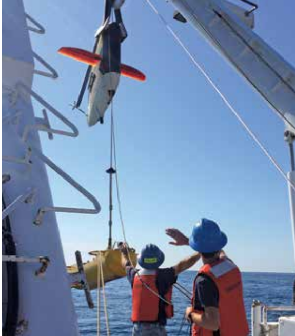
Professor Chris Roman's "wire flyer," an ocean sensing system designed to take measurements at varying depths in the water column, was deployed for testing. Photo: Lynne Butler
