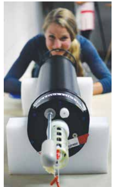
The author inspects an Argo float during an international ocean observing session led by Howard Freeland.
