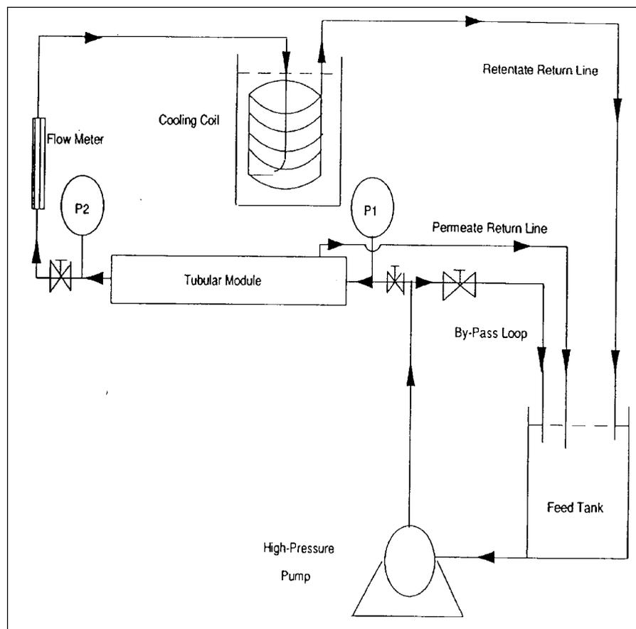
Fig. 2—Schematic of flow loop for a pilot scale UF/RO system. (P1 = inlet pressure gauge; P2 = outlet pressure gauge.)
