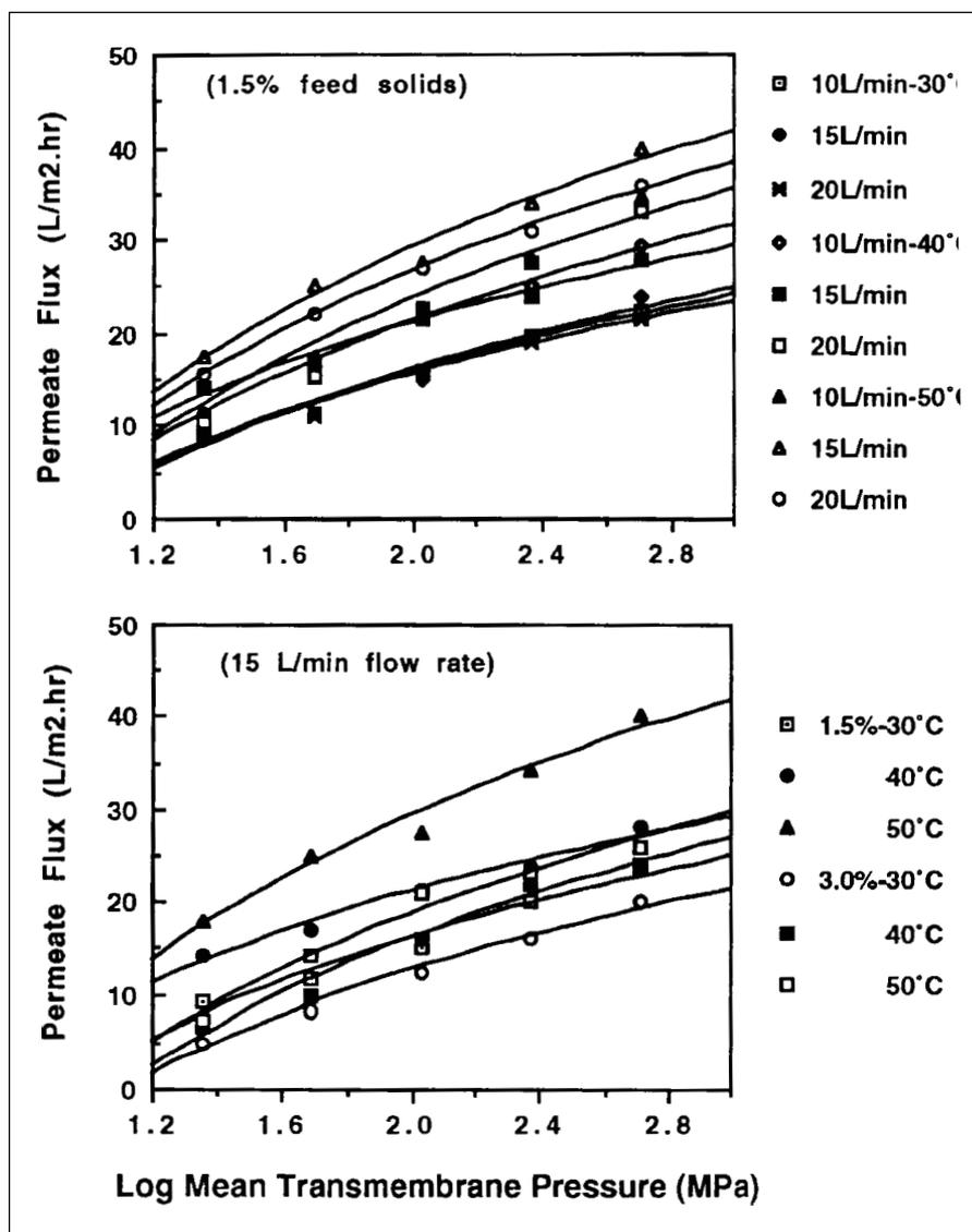
**Fig. 5—Changes in permeate flux of feeds with log mean transmembrane pressure in a pilot scale RO system at 1.5% feed solids with varying flow rates and feed temperatures, and at 15 L/min flow rate with varying feed solids and temperatures.**
