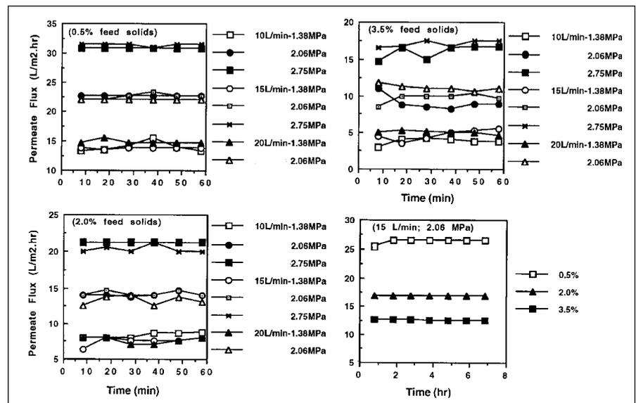
Fig. 3—Changes in permeate flux of feeds with time in a pilot scale RO system at 30°C feed temperature with varying feed solids, flow rates and transmembrane pressures.
