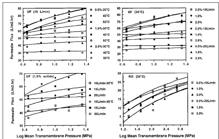
Fig. 4—Changes in permeate flux of feeds with log mean transmembrane pressure in a pilot scale UF and RO systems at varying feed solids and temperatures, and flow rates.
