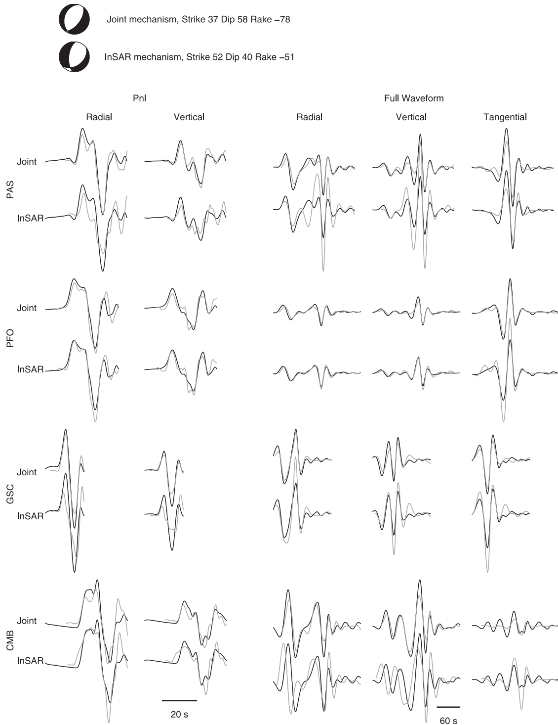
Figure 5. Mechanisms, observed waveforms, and synthetic waveforms from the joint and InSAR-only inversions using the Mojave layered model. Pnl waveforms are filtered from 0.01 to 0.2 Hz, while full waveforms are filtered from 0.01 to 0.05 Hz. Data are shown as solid lines and synthetics as shaded lines. The timescale is shown at the base of each group of plots, with the 20-s bar referring to the Pnl waveforms and the 60-s bar referring to the full waveforms.
