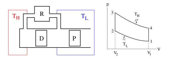
Piston P expands gas at high temperature  $T_H$  and compresses gas at low temperature  $T_L$ .
