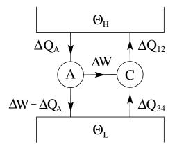
Heat transfers:  $\Delta Q_A > 0$ ,  $\Delta Q_{12} < 0$ ,  $\Delta Q_{34} > 0$ . Work performance:  $\Delta W = \Delta W_{out}^{(A)} = \Delta W_{in}^{(C)} > 0$ . Efficiencies:  $\eta_A = \frac{\Delta W}{\Delta Q_A}$ ,  $\eta_C = \frac{\Delta W}{|\Delta Q_{12}|}$
