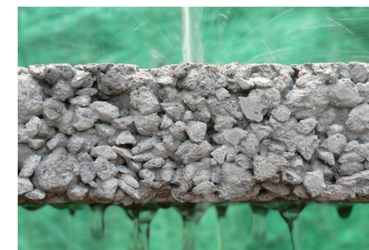
Figure 6: Pervious Concrete. Showing the infiltration capacity of the Pervious Concrete
