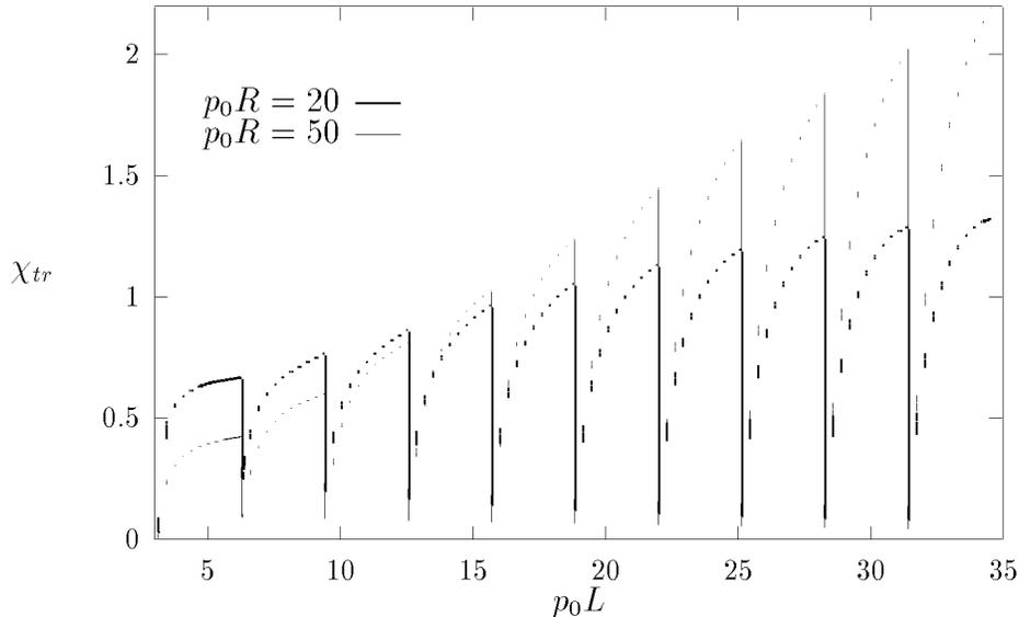
FIG. 6. Relative interference contribution to transport time,  $\chi_{tr}$ , Eq. (35), as a function of the film thickness  $p_0 L$  for  $p_0 \ell = 0.1$ ,  $p_0 \mathcal{L}_b = 20$ ,  $\tau_{tr}^b / \tau_b = 1.5$ , and two values of the correlation radius,  $p_0 R = 20; 50$ .
