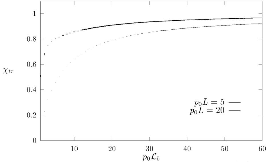
FIG. 5. Relative interference contribution to transport time,  $\chi_{tr}$ , Eq. (35), as a function of the bulk free path  $p_0 \mathcal{L}_b$  at constant ratio  $\tau_{tr}^b/\tau_b = 1.5$ . The inhomogeneities are characterized by  $p_0 R = 10$ ,  $p_0 \ell = 0.1$ ; the film thickness is  $p_0 L = 5; 20$ .
