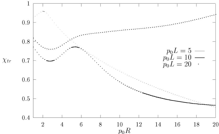
FIG. 4. Relative interference contribution to transport time,  $\chi_{tr}$ , Eq. (35), as a function of the size of the inhomogeneities  $p_0R$  for  $p_0\ell = 0.1$ ,  $p_0\mathcal{L}_b = 10$ ,  $\tau_{tr}^b/\tau_b = 1.5$ , and three values of the film thickness,  $p_0L = 5; 10; 20$ .
