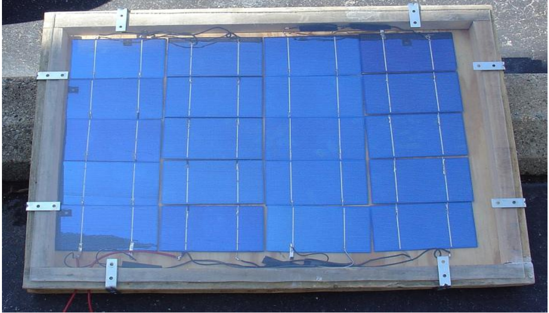
Figure 1.20 30W/2.5V solar panel
