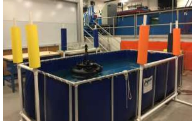
Figure 3. Actual tank configuration, utilizing 8 navigation aids for position calculation.
