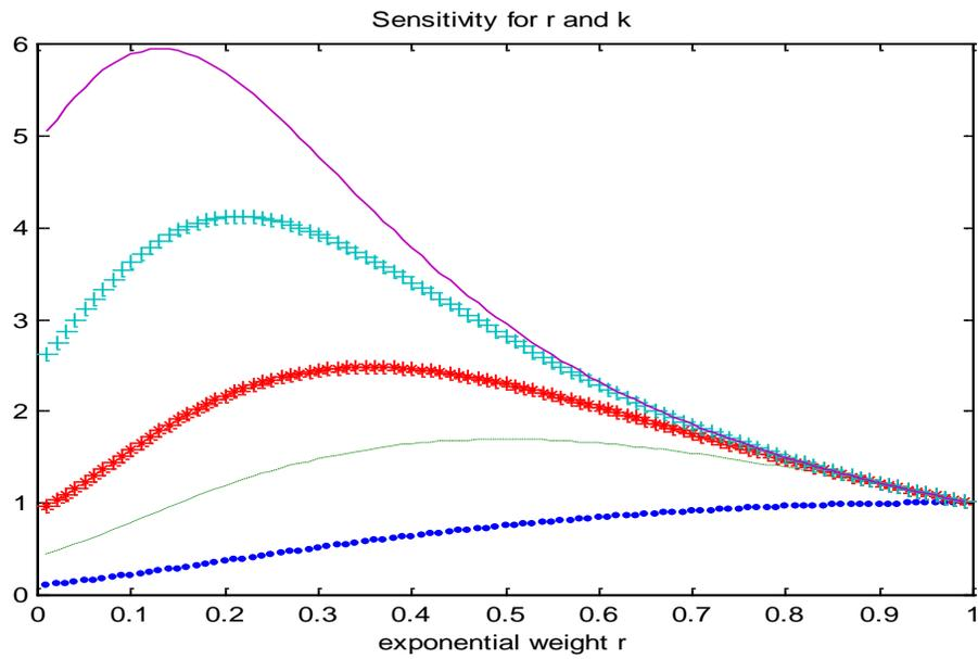
Figure 1 (c). The Sensitivity Factor  $S_{rk}$  for Mean Shift, small  $i$  ( $i=10$ )
