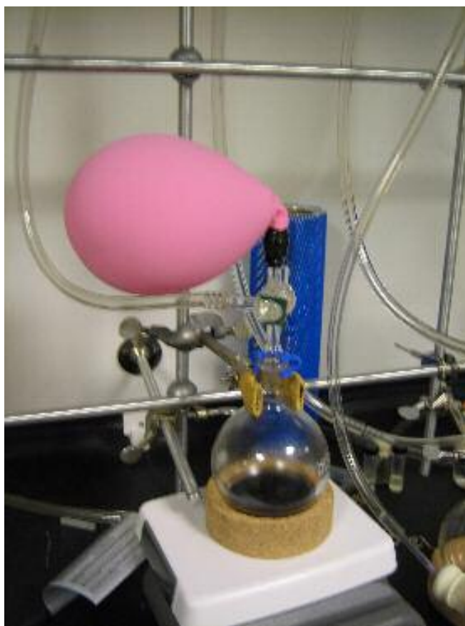
Figure 11. Hydrogenation Set Up. Balloon deflated slightly after a few hours. Photo by J. Lau.
