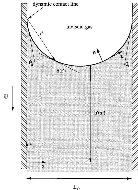
FIG. 1. The model system. A plate immerses into a contained bath of liquid of infinite depth at speed  $U$ . The right wall is stationary. The dynamic contact angle is  $\theta_D$  and the static contact angle is  $\theta_S$ . The hypothetical lower boundary restricts the computational domain.
