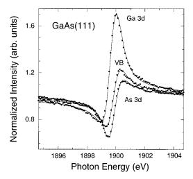
FIG. 3. Photon-energy dependence of the Ga 3d, the As 3d, and the GaAs valence-electron emission near the GaAs(111) Bragg back-reflection condition. The lines are the theoretical fits to the data points.
