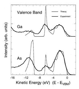
FIG. 13. Comparison of the *chemically resolved* Ga and As contributions to the GaAs valence band with the theoretically calculated Ga and As partial density of states. The upper portion of the figure shows the cation contributions, and the lower portion of the figure shows the anion contributions. The spectra have been offset for clarity. The solid lines are the experimental data, and the shaded lines are the theoretical calculations.
