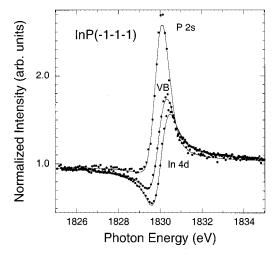
FIG. 6. Photon-energy dependence of the In 4d, the P 2s, and the InP valence-electron emission near the InP(-1-1-1) Bragg back-reflection condition. The lines are the theoretical fits to the data points.
