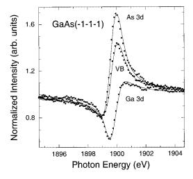
FIG. 4. Photon-energy dependence of the Ga 3d, the As 3d, and the GaAs valence-electron emission near the GaAs(-1-1-1) Bragg back-reflection condition. The lines are the theoretical fits to the data points.
