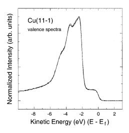
FIG. 10. Comparison of the high-resolution Cu valence-photoemission spectra. The spectra have been normalized to equal peak height and referenced to the Fermi energy. The large peak at intermediate binding energy arises from the Cu 3d contribution to the Cu density of states, while the emission near the Fermi energy is of 4s origin. The spectral line shapes are indistinguishable within the experimental uncertainties.
