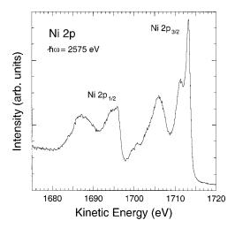
FIG. 11. High resolution Ni 2p core-photoemission spectrum from NiO.
