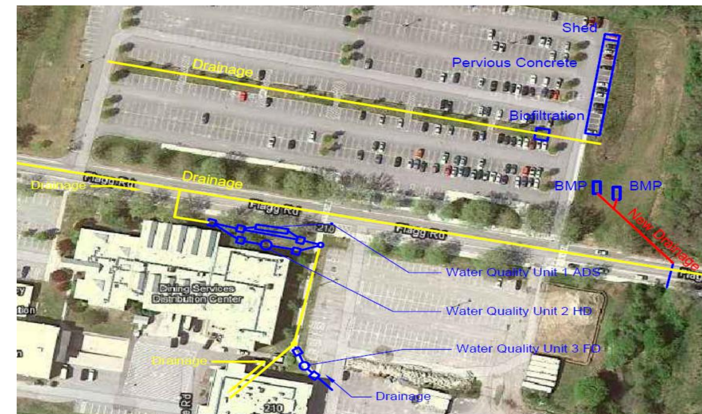
Figure 1: Schematic of the stormwater management and treatment demonstration facility (RI SDF) on the URI campus in Kingston, RI. There are two drainage systems to which BMPs can be connected to either the runoff generated on the surface of the parking lot (yellow) or from Flagg Road (red). Shown are the tentative locations for the hydraulic separator and the pervious pavement. Also shown are the tentative locations of other treatment structures, such as a biofiltration unit and another BMP.
